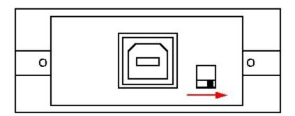
When data logging on any other vehicles, this switch should be set towards the USB connector.
