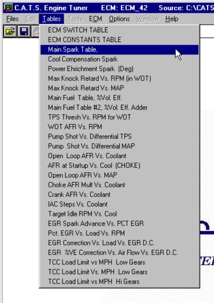
To make the calibration tables easy to understand and more convenient to edit, the C.A.T.S. Tuner program displays all table values in correct engineering units rather than the binary values actually stored in the calibration file.
