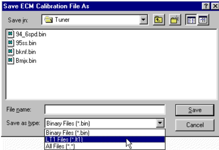
Before saving the ECM calibration file, the program recalculates the necessary checksums and builds a valid ECM calibration file that can be used to program an EPROM for the ECM.
