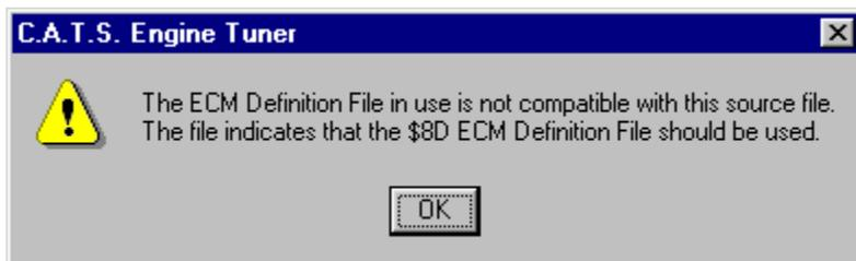
To open the selected calibration file, note which definition file is indicated and click the 'OK' button. Click on the 'ECM' drop-down menu and select the correct ECM Definition File (if installed) and then re-open the desired calibration file.
