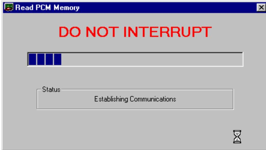
The progress meter shows the progress on the reading of the PCM as it proceeds and the Status window describes what part of the process is currently underway. Depending on the PC you are using, the programming will usually take about five minutes. If the process does not complete correctly for some reason, an error message will be displayed in the Status window. See Appendix B for a description of the possible error messages.
