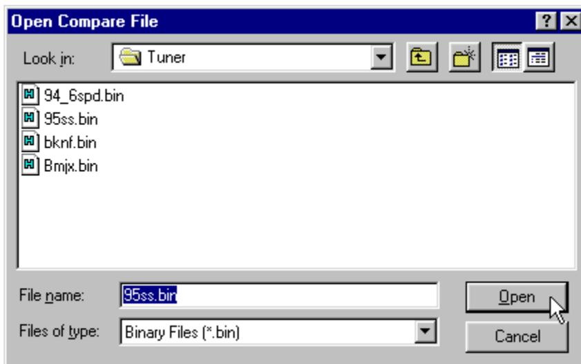
If you are using the \$EE ECM Definition File, the Tuner program will accept .lt1 format files as well as standard binary format files as compare files. You can even compare an .lt1 file to a binary file.
