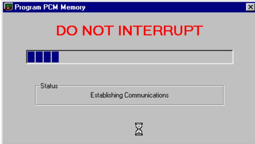
The progress meter shows the progress on the programming as it proceeds and the Status window describes what part of the process is currently underway. Depending on the PC you are using, the programming will usually take about five minutes. If the process does not complete correctly for some reason, an error message will be displayed in the Status window. See Appendix B for a description of the possible error messages.
