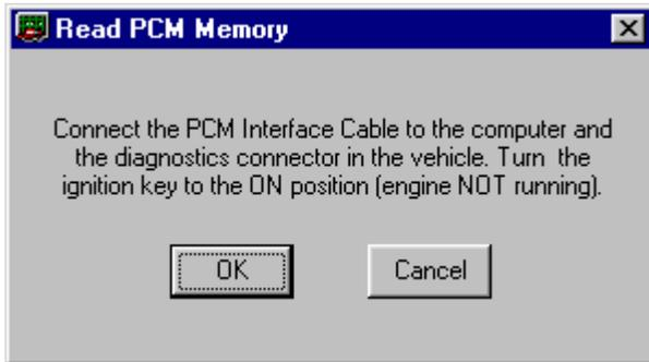
Before proceeding, connect the RS-232 to ALDL converter interface cable to the Comm port on your PC. If your PC has more than one Comm port, make sure you connect the converter to the com port that you specified on the Comm Port Setup screen.
