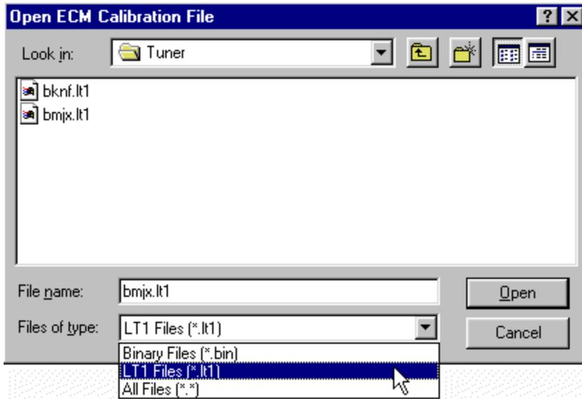
When you select a calibration file, the program will verify that it is a valid calibration file and that the correct ECM Definition File has been selected. If the incorrect configuration file has been selected, the following error message will be displayed. If possible, the program will indicate which ECM Definition File is required for the selected calibration.
