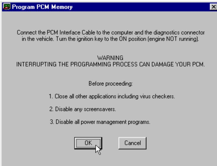
Before proceeding, connect the RS-232 to ALDL converter interface cable to the Comm port on your PC. If your PC has more than one Comm port, make sure you connect the converter to the Comm port that you specified on the Comm Port Setup screen.
