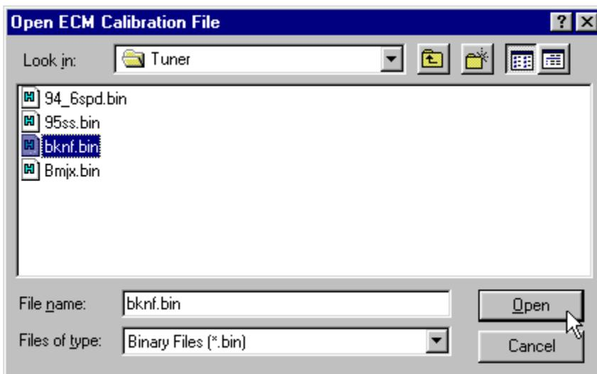
If you are using the \$EE ECM Definition File, the Tuner program can also open .lt1 format files.
