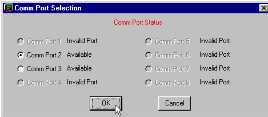
This screen allows you to select which comm port on your PC will be used when communicating with the PCM for reading and programming the PCMs FLASH memory. To select the desired comm port, click on that port and then click 'OK'.
