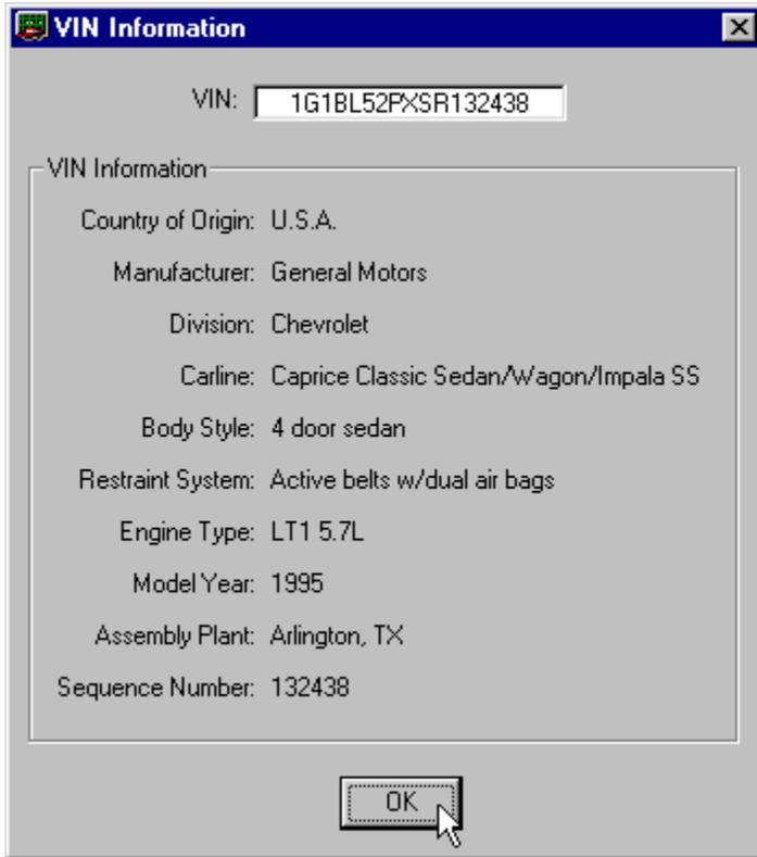
Note: The actual VIN is stored in EEPROM on the microprocessor and cannot be changed by editing the copy that appears in the calibration file from the FLASH memory.
